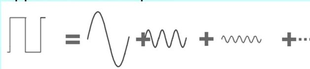
$$u(t) = 4U/\pi (\sin \omega t + 1/3 \sin 3\omega t + 1/5 \sin 5\omega t + \dots)$$
